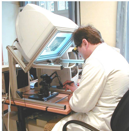
Figure 6: Configuration of the simulator for virtual petrous bone surgery: the position of the surgeon's hands, patient orientation and viewing direction similar to the real procedure and spatial perception is enhanced by stereoscopic viewing.
