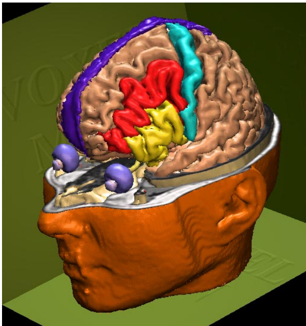
Figure 17: Object rendering using attribute interpolation only (compare with fig. 7). Objects with high curvature look very similar while areas with low curvature such as the skin surface reveal some artifacts.
